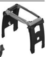
Fully unfold legs to position shown above and hand-tighten the four plastic fasteners.
